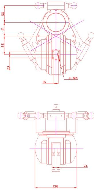
基座安装 Base installation (mm)
