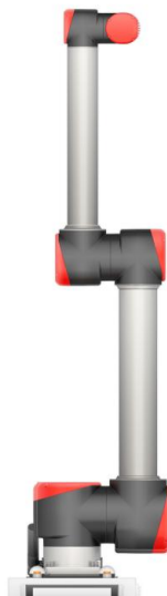
Figure 1.12 mechanical zero point position diagram1
